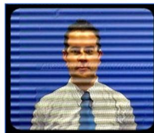
The reason for the problem is that high pressure weather systems can cause signals to travel long distances with ease. This means that as well as your local transmission, your aerial can pick up those from distant transmitters as well. If they are on the same frequency, the result is co-channel interference.
