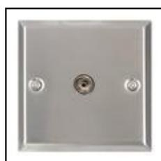
The quality of wall-mounted aerial outlets can have an effect on reception. Those with a screened metal plate are preferred for digital TV, and if signals are known to be marginal, use satellite-grade double-screened co-axial cable for the lead between your aerial outlet and your equipment. Also use metal RF plugs rather than plastic ones.
